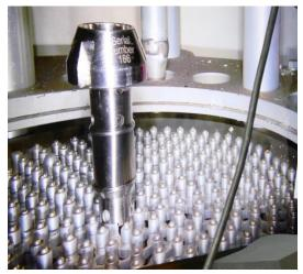
Fig. 4. The adapter pintle installed on the core
