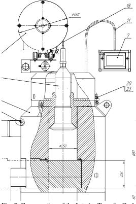
Fig. 3. Cross section of the Interim Transfer Cask
